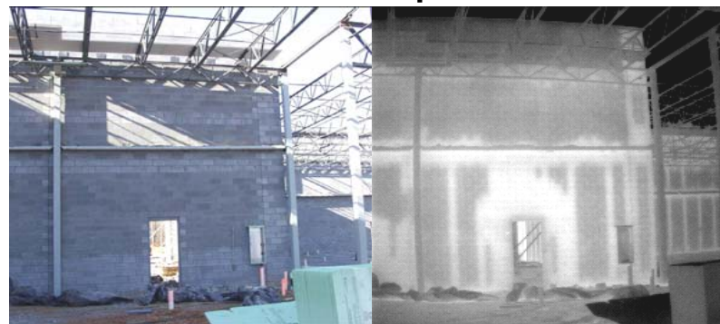
“See” the foamed-in-place insulation.
